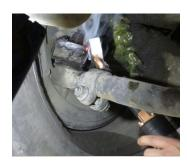
Wide range of inductors designed to provide maximum power. The flux concentrator and the protective cap resistant to high temperatures are blocked without glue.
